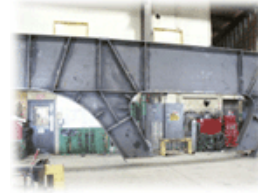
Complex "Haunched" Welded Plate Highway Bridge Girders
